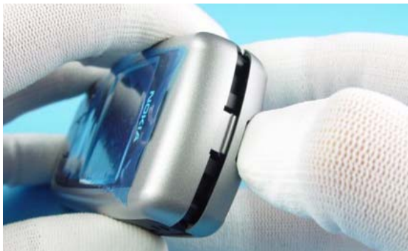
3) Press the A-Cover Lock before removing the B-Cover
