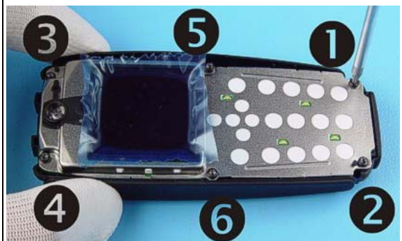
6) Remove screws by using the shown order.
