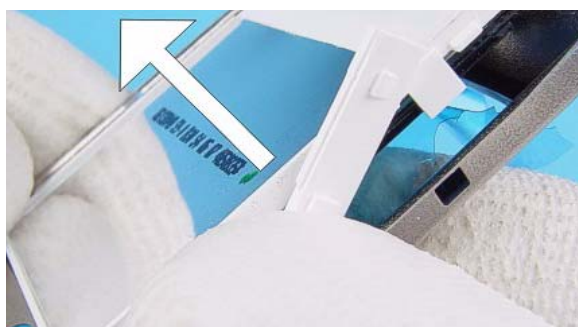
11) Press out the LCD Module while bending the C-Cover gently.
