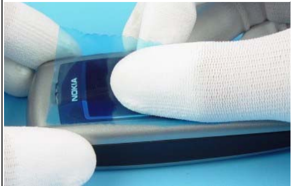
2) Protect the Window with a protective film.
