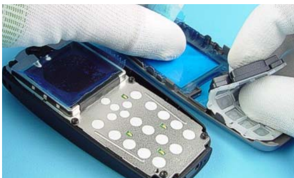
5) Remove Keypad, protect LCD and inner side window with a protective film.
